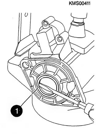
Checking drive-end bearing
